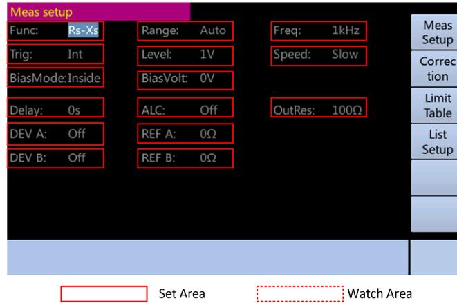
In the measurement setup page, the user can move the cursor to the corresponding field to configure all of the following measurement control functions.
